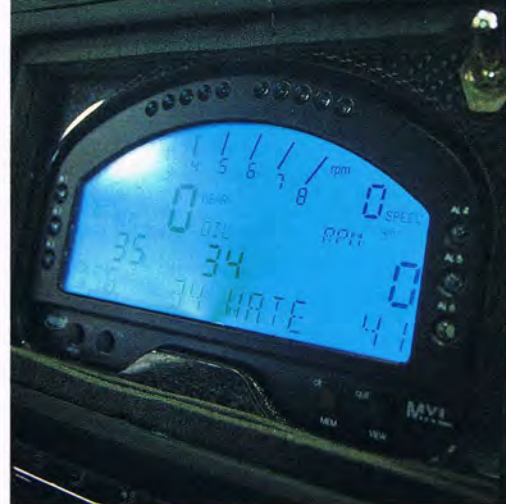
AIM data logging system fits snugly where stereo
